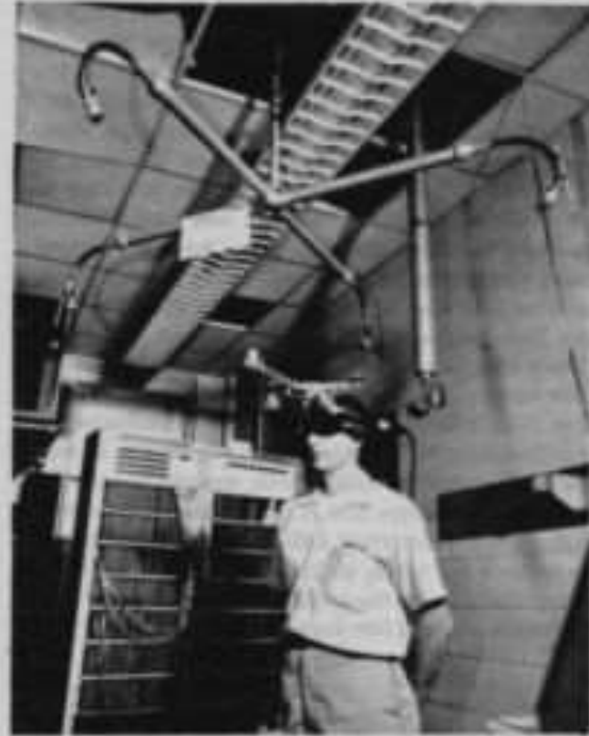
FIGURE 5--The mechanical head position sensor in use
